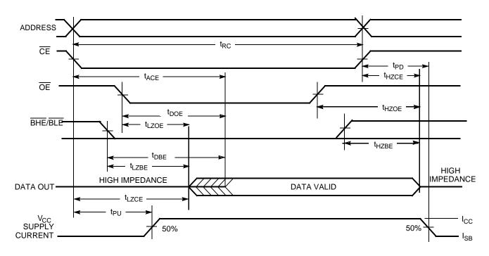
Notes:15. The device is continuously selected.  $\overrightarrow{OE}$ ,  $\overrightarrow{CE} = V_{IL}$ ,  $\overrightarrow{BHE}$  and/or  $\overrightarrow{BLE} = V_{IL}$ .16. WE is HIGH for read cycle.17. Address valid prior to or coincident with  $\overrightarrow{CE}$  and  $\overrightarrow{BHE}$ ,  $\overrightarrow{BLE}$  transition LOW.
